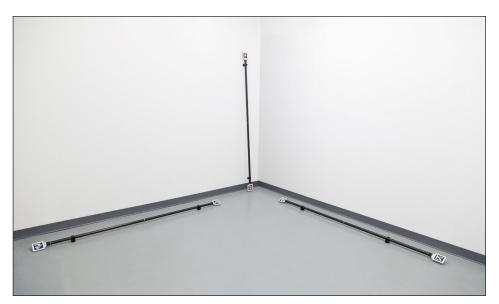
Scale bars may be assembled to establish scale for x, y, and z, as shown left, or in different configurations to meet specific project needs.
