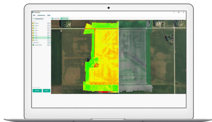
Pix4Dfields comparison tool (split screen) showing a NDRE index map on the left and an orthomosaic on the right.
